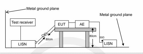
LISN: Artificial Mains Network AE: Associated equipment EUT: Equipment under test
